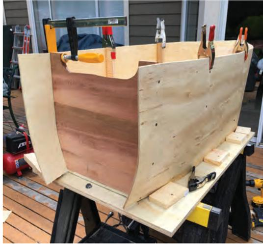
3. 1 - 4'x8' 1/4" Plywood (Sides of Boat) - Cut to 20"x60".
