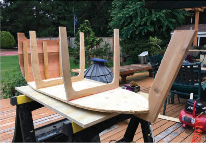
1. 1 - 4'x8' 3/4" Plywood (Base of Boat) – Shape and trim to bow shape
