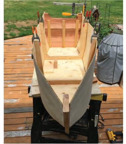
5. Use clamps, glue and screw plywood together.
